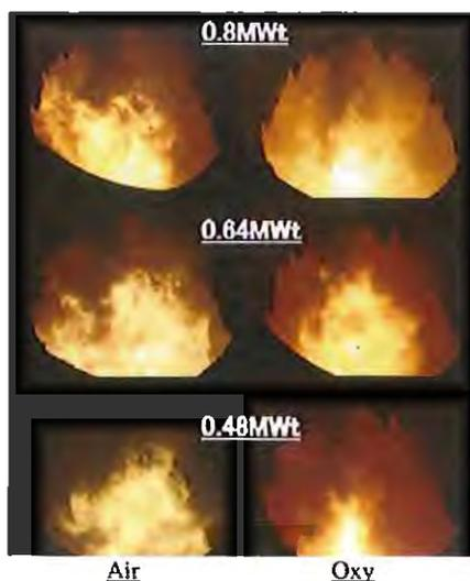
Fig.4 Photos of flame at air and oxy combustion on Coal B
