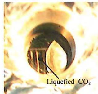
Fig.3 Photo of captured CO<sub>2</sub> in the liquefaction
