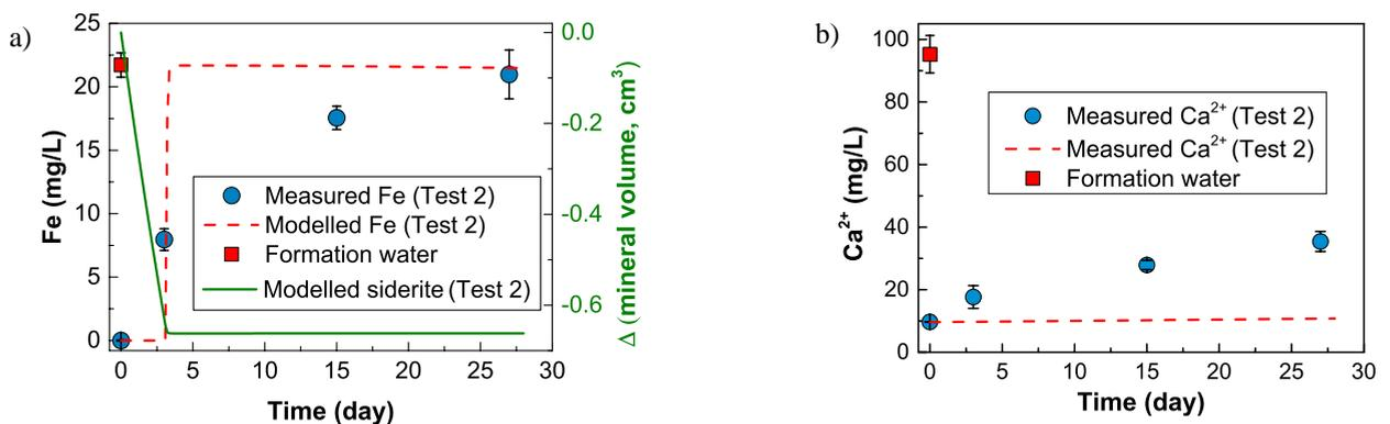
Fig. 4. Measured and predicted concentration of (a) total Fe and (b) Ca<sup>2+</sup> in the back-produced water in Test 2.
