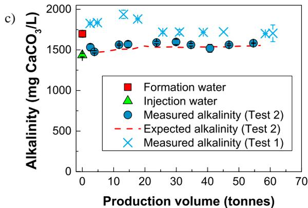
Fig. 3. Measured and expected concentration of Ca<sup>2+</sup> and total Fe (a and b) and measured and expected total alkalinity in the back-produced water in Test 2 (c).
