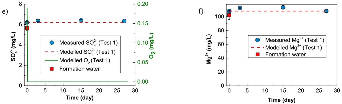
Fig. 2. Measured and predicted concentration of (a) total Fe, (b) Si, (c)  $\text{K}^+$ , (d)  $\text{Ca}^{2+}$ , (e)  $\text{SO}_4^{2-}$  and (f)  $\text{Mg}^{2+}$  in the back-produced water in Test 1.
