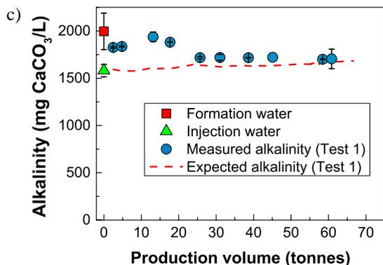
Fig. 1. Measured and expected concentration of  $\text{Ca}^{2+}$  and total Fe (a and b), and measured and expected total alkalinity in the back-produced water in Test 1 (c).
