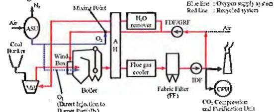
Fig.3: Combustion system flow on Callide Oxyfuel Project
